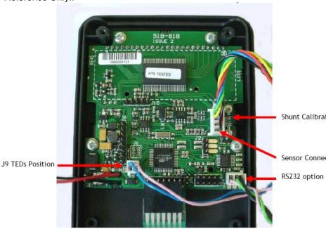
Shunt Calibration Resistor
