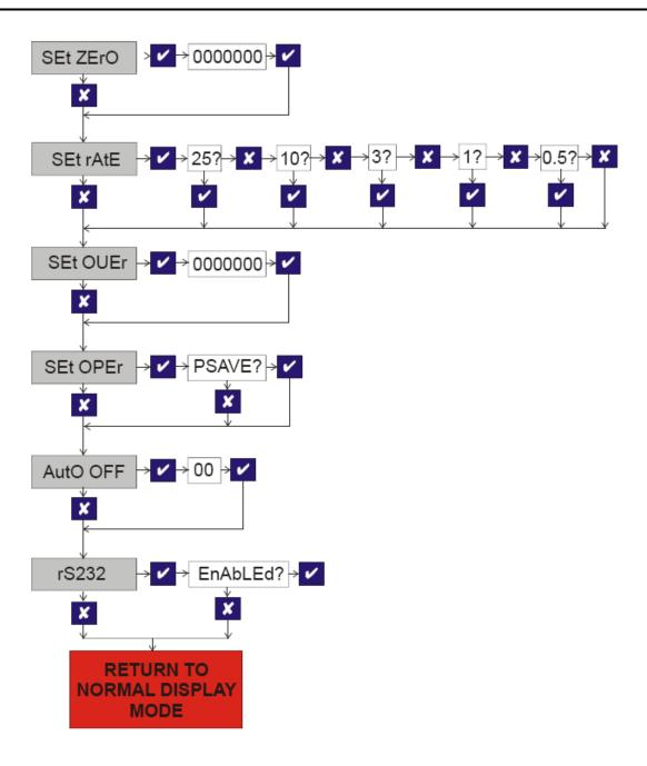
The CALIBRATION MENU is used to calibrate ranges with independent scales and to set the display resolution for each range.
