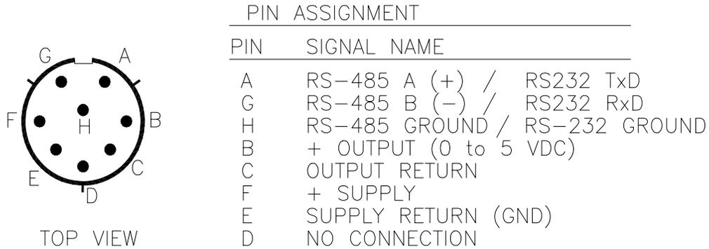
**Figure 7.1 Electrical Connector Pin Assignments**
