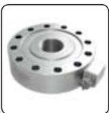
**Intrinsically Safe Coiled Tubing Load Cells:** Low profile tension / compression load cells for mounting on coiled tubing injector stands. Features high level electrical output and noise immunity • Potential applications include monitoring tubing weight and insertion force, as an electronic replacement for a hydraulic load cell, and monitoring footpad loads of injector head jackstands
