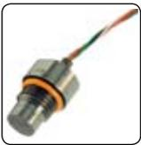
**MWD Miniature Pressure Sensors:** Compact size and stainless steel construction, designed to measure pressure ranges up to 30,000 psig and operating temperatures up to 400 °F • Potential applications include measurement while drilling, monitoring pressurized tools, and mud pulsation
